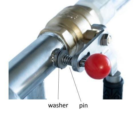
Caution: Never put air pressure in the device without the locking pin securely in place
