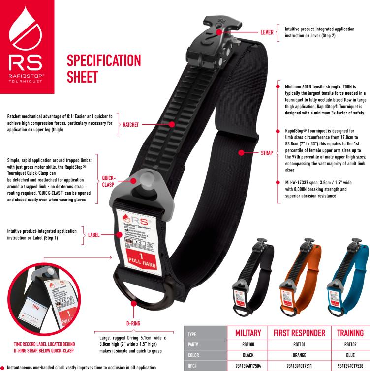
Instantaneous one-handed cinch vastly improves time to occlusion in all application scenarios. Easy and quick to apply; requires no stabilizing hand and supplies a mechanical advantage of 2:1 prior to effecting tightening mechanism
