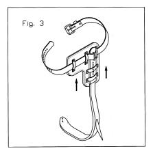
Slide the climber pad along the shank of the climber onto the sleeve, aligning the sleeve loop with the loops on the horizontal leg of the pad. Insert climber strap in the direction shown, through the pad loops and the climber sleeve loop. See Fig. 3 ('right' climber shown). Note: Foot strap must be attached to the leg iron stirrup in the same direction as shown for the calf strap.
