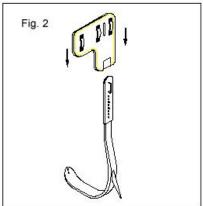
Slide the climber pad along the climber sleeve onto the climber, aligning the sleeve loop with the loops on the horizontal leg of the pad. Insert climber strap in the direction shown, through the pad loops and the climber sleeve loop. See Fig. 3 ('right' climber shown). Note: Foot strap must be attached to the leg iron stirrup in the same direction as shown for the calf strap.
