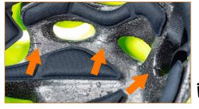
Internal polystyrene shell broken in several places.
