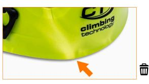
General deformation of the shell: material shows signs of having been weakened.
