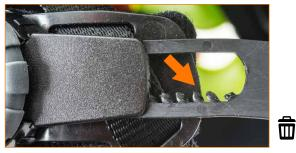
Headband adjustment mechanism has damaged teeth and doesn't stay in position.
