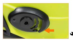
Visor support broken. Replace with suitable spare part..
