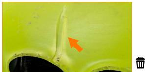
Shell shows impact damage in one place.
