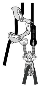
Rock Exotica recommends separating the Akimbo and termination end of the rope. The Rock Exotica Hydra is one example of a suitable connection. Connect the Akimbo using an appropriate oval carabiner. Rock Exotica recommends a RockO WireEye carabiner
