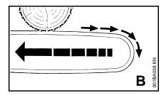
When the chain on the top of the bar – underbucking – is suddenly pinched, caught or encounters a foreign object in the wood, the chain saw may suddenly be driven straight back toward the operator – to avoid this:
