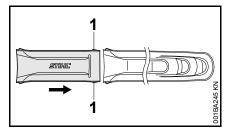
Push the scabbard extension and chain scabbard together – the lugs (1) must engage in the chain scabbard.
