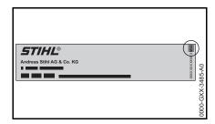
The STIHL M-Tronic version is indicated on the approval label of the chain saw, e.g. "M3.0" indicates the STIHL M-Tronic version 3.0.
