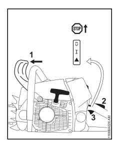
Push the hand guard (1) forward – the chain is locked.
