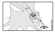
Use the plunge-cutting sight if possible. The plunge-cutting sight and the top and bottom of the guide bar are parallel.
