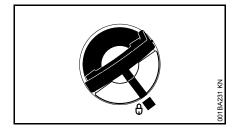
The marks on the tank cap and fuel tank are then in alignment.
