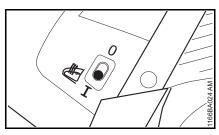
Set switch to I – to switch off, return switch to the 0 position
