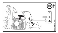
• If the engine was started in the start position ▲: Press down trigger lockout and the pull the throttle trigger (2) at the same time – the Master Control lever (1) moves to the run position (I) and the engine settles down to idling speed.
