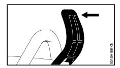
Pull hand guard towards the front handle until it engages audibly – chain brake is released
