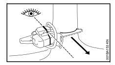
Position the saw in the horizontal cut. The gunning sight must point in the planned direction of fall – if necessary, correct direction of fall by re-cutting the felling notch.
