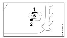
Turn screw (1) to the left until the tensioner slide (2) butts against the left end of the housing slot
