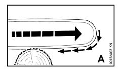
When the chain on the bottom of the bar – overbucking – is suddenly pinched, caught or encounters a foreign object in the wood, the chain saw may suddenly
