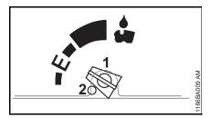
The oil flow can be adjusted as needed using the adjusting screw (1) (on the bottom of the machine).
