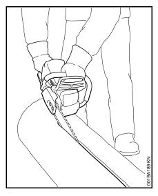
Cutting technique in which the spiked bumper is not used – risk of pull-in – start the cut with the guide bar at the shallowest possible angle – take extra care since there is an increased danger of kickback.
