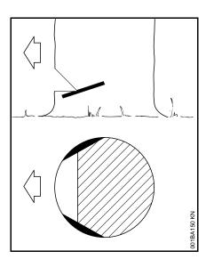
Sapwood cuts in long-fibered softwood help prevent sapwood splintering when the tree falls. Make cuts at both sides of the trunk at same height as bottom of felling notch to a depth of about 1/10 of trunk diameter. On large diameter trees, cut to no more than width of guide bar.
