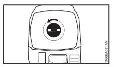
Turn the knob above the rear handle in the direction of the arrow and remove the carburetor box cover
