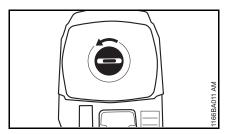
Turn the cap above the rear handle in the direction of the arrow and remove the filter cover
