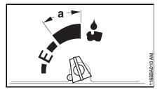
If necessary, the oil flow can be increased beyond the standard setting.
