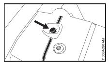
Press in the button to open the decompression valve.
