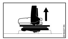
Remove the tank cap.
