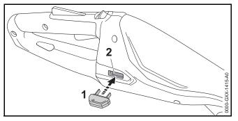
Insert the activation key (1) in the socket (2).
