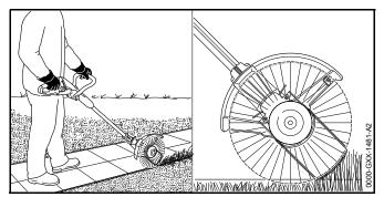
Guide the trimmer along the edge of the lawn. The bump guard maintains the required ground clearance.
