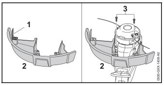
The line limiting blade (1) is already installed in the deflector (2) and must not be removed.
