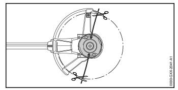
► Cut the mowing lines so that they extend as far as the line limiting blade.
